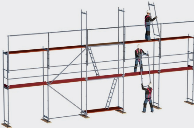
Figure 25: Example of vertical transport by hand
