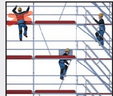
Only use fitted ladders or stairways for ascent and descent
