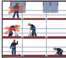
Workplaces may not be located above one another at any one time
