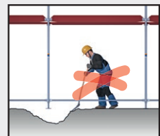
Do not endanger the stability of the scaffolding by excavating or digging around the base
